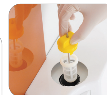
Bucket filter: Without dirtying the hands, the suction filter can be cleaned.
